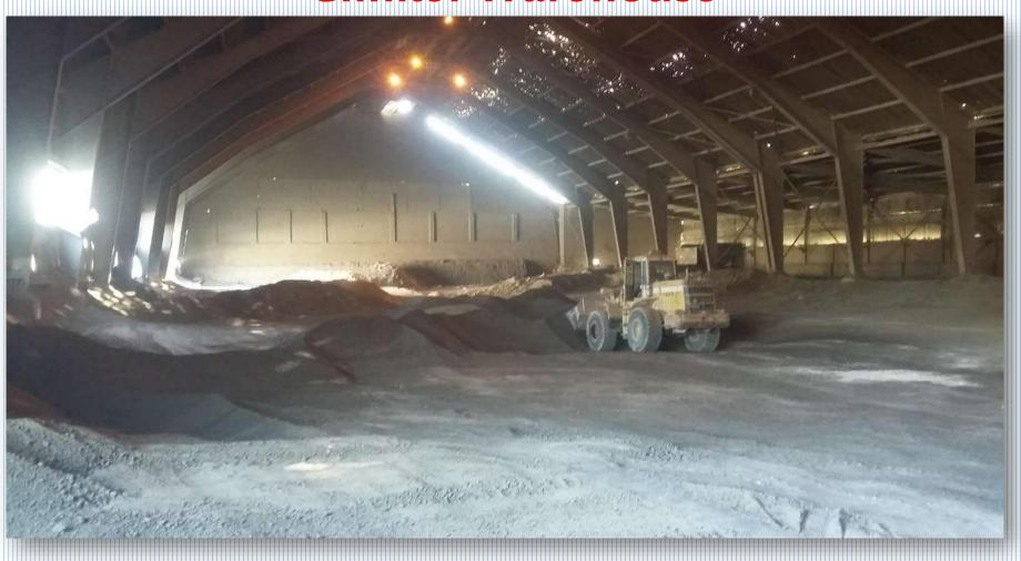
The clinker shall be handled through a loader, where the clinker is transferred inside a mobile hopper of 14 m<sup>3</sup> capacity and equipped with a conveyor belt for unloading.
